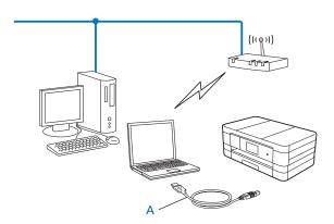
You can configure the wireless settings of the machine using a USB cable temporarily connected to a wired or wireless computer.
